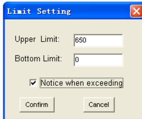
Selecting “Notice when exceeding” means that the over limit prompt function is enabled. Then, enter the required upper and lower limits respectively. If over limit prompt function is enabled, the measurement data that is over the limit will be displayed in red (graphic section).
