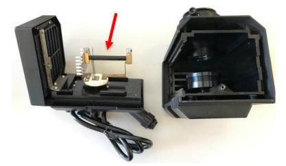
6. Loosen the two fixing screws at both ends of the HBO lamp.
