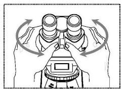
eyepieces completely overlap each other, i.e. they combine to form a circular image, then the interpupillary distance is set correctly.
