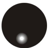
3. Adjust the height of the condenser until the image from the field diaphragm appears clearly in the field of view. For some microscopes there is a risk that you will lift the condenser up so high that it collides with the object holder. Therefore care is needed when doing this.
