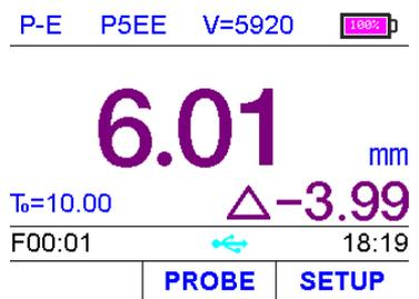
Although the gauge is excellent for single point measurements, it is sometimes advisable to examine a larger area and search for the point with the smallest thickness. The gauge has a "Scan Mode" function that enables it.
