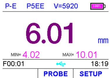
**Diff Mode.** Both the last thickness reading and the differential thickness value are displayed (of the absolute thickness value and the nominal thickness value).
