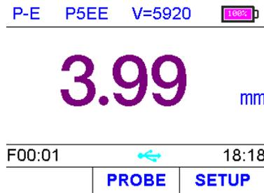
**Scan Mode** [*Scan Mode*]. In addition to the last thickness value measured, the minimum and maximum thickness values are also displayed during the measurement. By pressing
