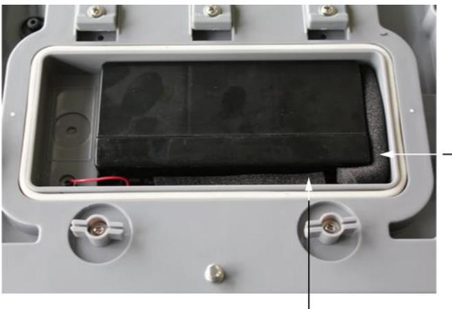
⇒ Insert the rechargeable battery in a manner that it cannot slip (fasten with a rubber foam mat)
