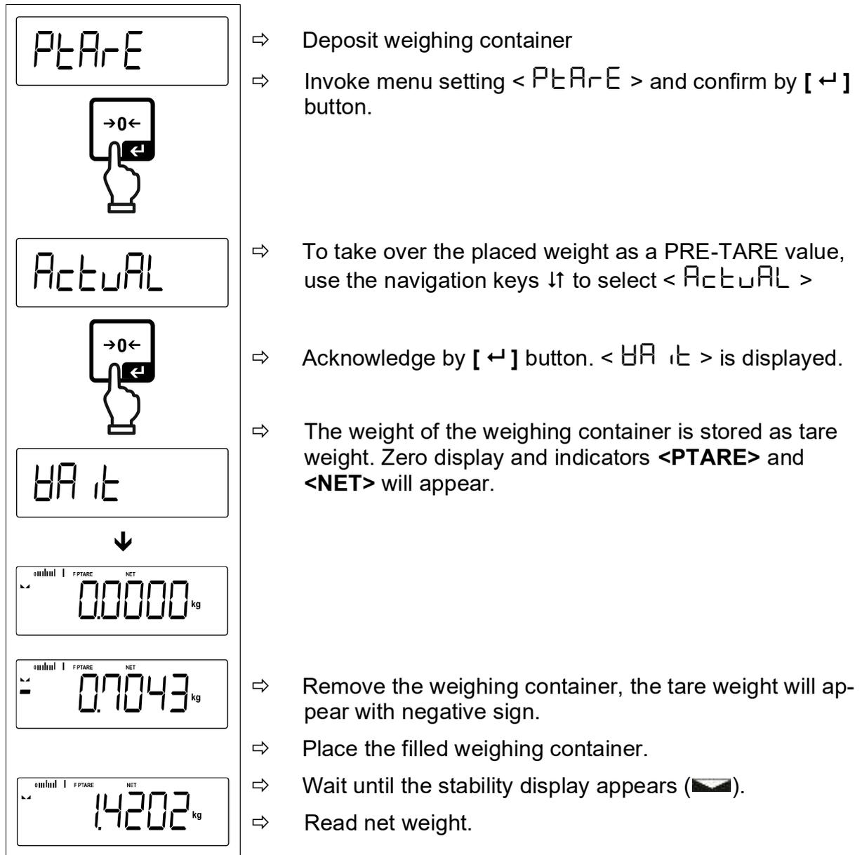
**i** The entered tare weight remains valid until a new tare weight is input. To delete press the TARE key or confirm the menu setting < C L E A R > using the [ ← ] button.
