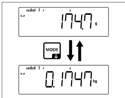
⇒ Using **[MODE]** button, it is possible to switch over between the enabled unit 1 and unit 2.
