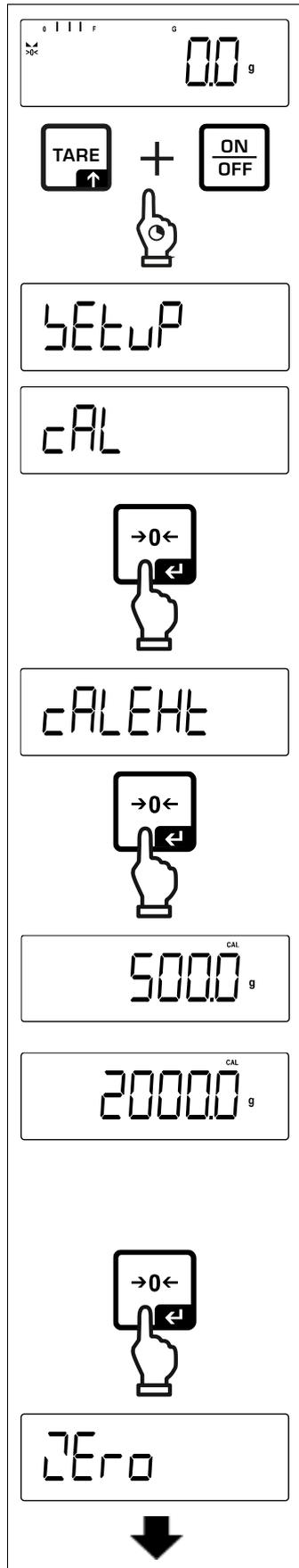
⇒ Press and hold the TARE and ON/OFF buttons simultaneously to enter the setup menu.
