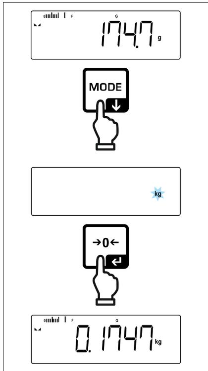
The unit for quick selection can be determined when the **[MODE]**-button is shortly pressed for the first time.
