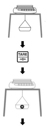
Attach empty immersion basket to hooks for underfloor weighing.
