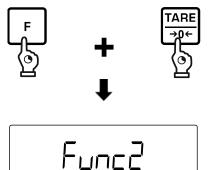
Press [F]- key and [TARE/ZERO] key simultaneously for about 2 seconds.
