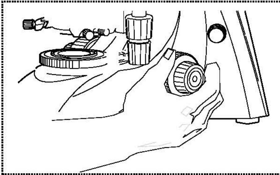
The simplest method for this would be to bring the stage (also using the coarse drive) to just below the lens beforehand and then slowly lower it. As soon as an image (no matter how sharp) can then be seen, the correct sharpness should only be set with the fine drive.
