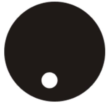
4. Using the centering screws of the condenser carrier, bring the image of the field diaphragm into the center of the field of view.
