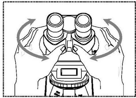
As soon as the field of view of the left eyepiece and the field of view of the right eyepiece overlap completely, or merge into a single circular image, the correct interpupillary distance has been set.
