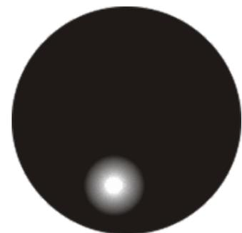
3. Adjust the height of the condenser until the image of the field diaphragm appears sharp in the field of view. With some microscopes, there is a danger of raising the condenser too high and causing a collision with the specimen slide. A little caution is therefore required here.
