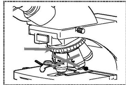
If you have focused the object of observation for a certain magnification, the focus can easily get out of focus when selecting the objective with the next higher magnification. In this case, the focus must be restored by slightly adjusting the fine adjustment knob.
