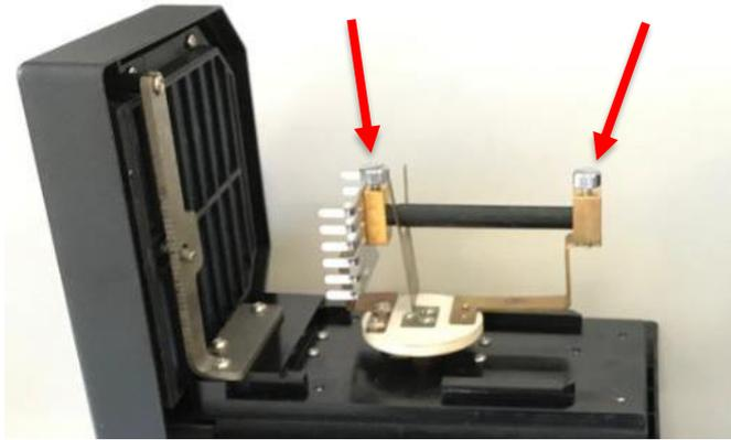
7. Replace the defective lamp or the transport fuse with a new lamp.
