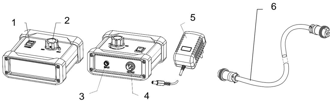
5W LED Power Box (front) DC input LED Power Box (rear) DC input LED power cable
