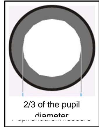
The view in the tube without the eyepiece should look something like the illustration on the right. The diameter of the aperture diaphragm which is then visible should make up approximately  $2/3$  of the pupil diameter.
