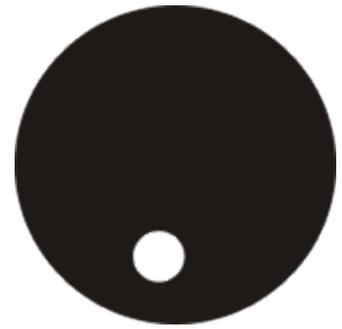
4. Use the centring screws of the condenser holder to bring the image from the field diaphragm into the centre of the field of view.
