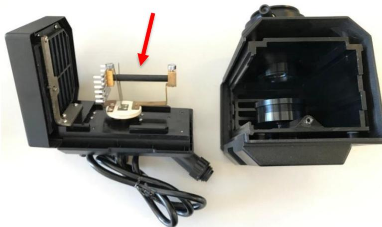
6. Loosen the two fixing screws at both ends of the HBO lamp.
