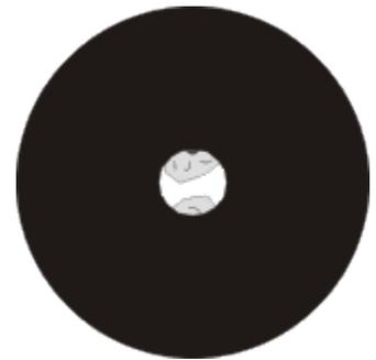
5. Open the field diaphragm until it just disappears out of the field of view. If necessary, simply re-centre using the centring screws on the condenser holder.
