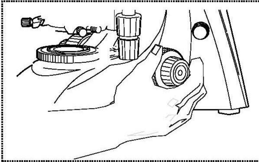
The simplest way of doing this would be to first raise the specimen stage (using the coarse adjustment knob) until it is just under the objective and then lower it slowly. As soon as an image is recognisable (no matter how sharp), then you should only adjust the focus using the fine adjustment knob..
