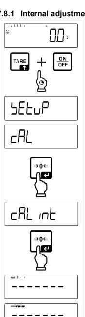
⇒ Press and hold the TARE and ON/OFF buttons simultaneously to enter the setup menu.
