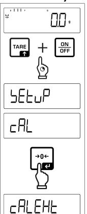
⇒ Press and hold the TARE and ON/OFF buttons simultaneously to enter the setup menu.
