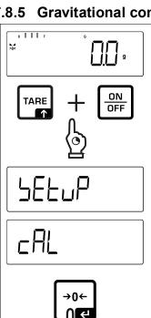
⇒ Press and hold the TARE and ON/OFF buttons simultaneously to enter the setup menu.
