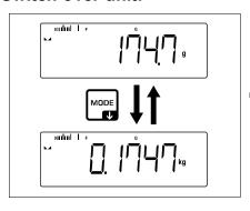
⇒ Using **[MODE]** button, it is possible to switch over between the enabled unit 1 and unit 2.
