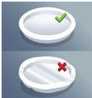
Always use KERN one-way sample trays. The measurement results very often turn out irreproducible if sample trays are reused.
