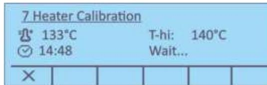
7. Temperature calibration for the second point takes 15 min. Compare the temperature displayed on the DLB-A01N with that of the moisture analyzer.
