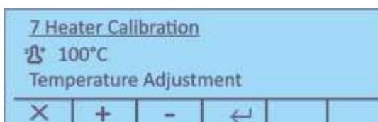
6. Confirm by
