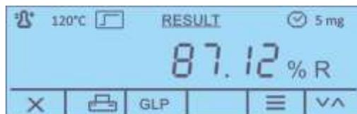
The dry material content (DC) of the sample will be displayed in percentages of the wet weight (=initial weight)
