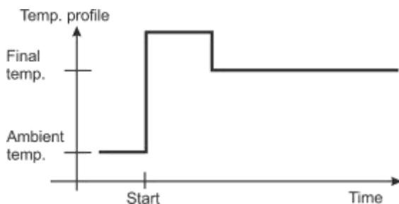
Quick drying is first and foremost suitable for samples with a moisture content of more than 30%. After start-up the temperature will be rising fast and exceed the set drying temperature by approx. 30% for about two minutes. This compensates the evaporation coldness and that way the drying process will be accelerated.
