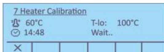
5. Temperature calibration for the first point takes 15 min. Compare the temperature displayed on the DLB-A01N with that of the moisture analyzer.
