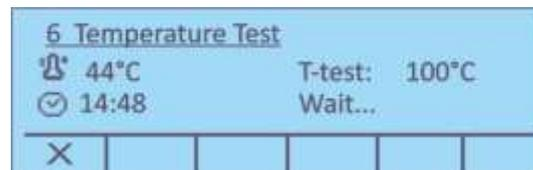
5. After 15 minutes the test is finished, an acoustic signal sounds. Compare the test temperature with the displayed temperature of the DLB-A01N. If the two values do not match, we recommend a temperature adjustment, see chap. 8.2.2
