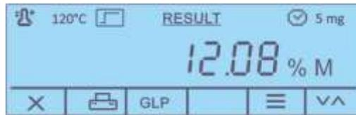
The moisture content of the sample will be displayed in percentages of the wet weight (= initial weight).
