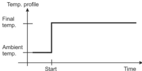
This heating profile is suitable for most samples. The sample is heated to the set temperature at normal output and is then kept at this temperature.
