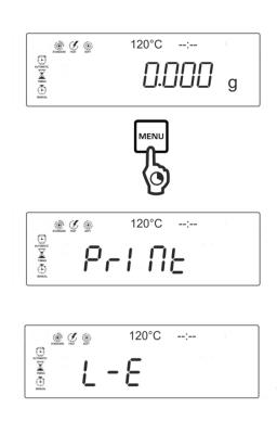
Acknowledge with . The protocol of the measurement carried out as last is displayed under the ident number "1". The instrument stores the last five protocols (ident number 1 -5). With every new measurement, the ident number One will be overwritten.
