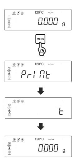
This is the starting/finishing time of continuous data transmission when the measurement is started/completed.
