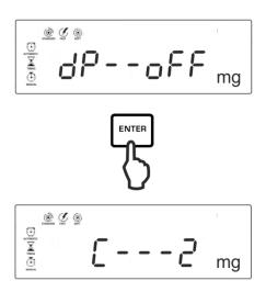
Press to confirm and set the required data transmission cycle using the navigation buttons (you can select from: 1, 2, 5, 10, 30, 60, 120, 300, 600 s).
