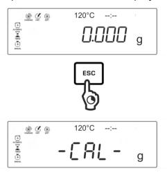
⇒ Wait until the weighed value for the required adjustment weight appears flashing.
